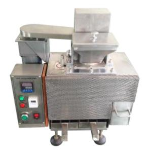
The Optimum SS12M Solder Dross Separation Machine has been designed to efficiently separate solder from solder dross by means of a regulated heated chamber and a high-speed rotor reclaiming up to 80% of the solder.
