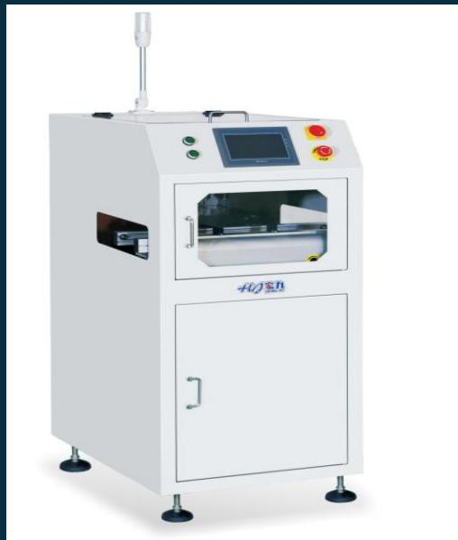
The Vacuum loader machine is used to store stacked PCB,s at the start position of the SMT production line – On request an individual PCB will be picked up by vacuum and transferred to the preceding in line conveyor/Screen printer
